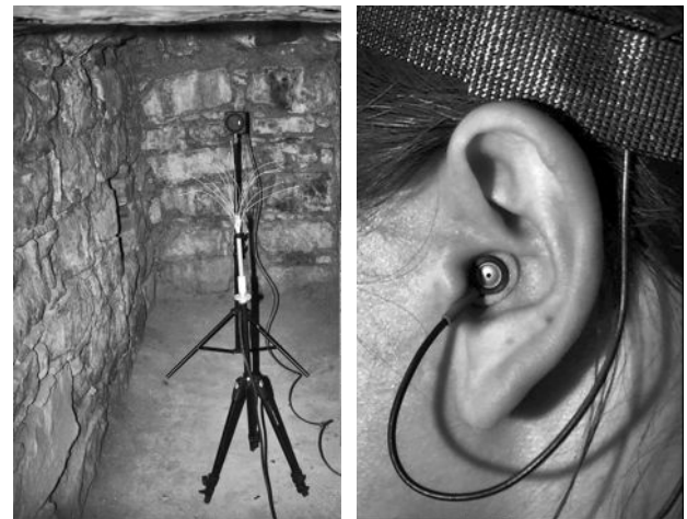
Fig. 11 Acoustic measurement equipment used in Chavín galleries: (a) 4" single-driver loudspeaker (Meyer MM-4XP) and the "bouquet" microphone array designed by our team (Countryman B6 elements); (b) Binaural recording employs omnidirectional microphones (Sennheiser/AuSIM) positioned in the outer ear canals of a researcher. Photos by José Luis Cruzado Coronel.
